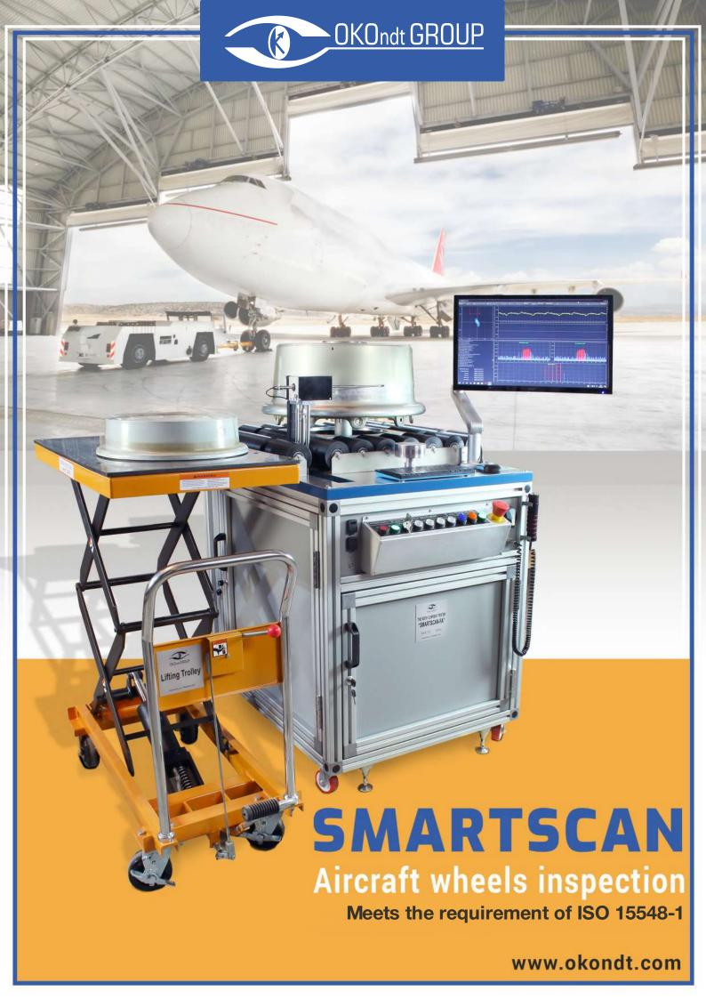
**SMARTSCAN Aircraft Wheel Inspection** System is intended for testing of main and nose wheels of aircrafts of various world manufacturers such as Messier - Bugatti, Goodrich, Honeywell, Maggitt and others.
